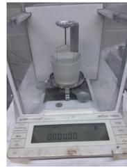
Figure 2: Density apparatus.
