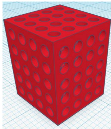
Figure 2: Foam CAD model (56.9% porosity)
