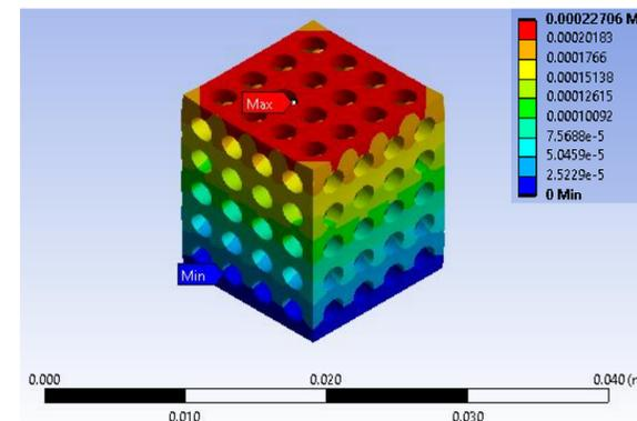
Figure 4: Simulated compression test of Mg foam, deformation (mm)
