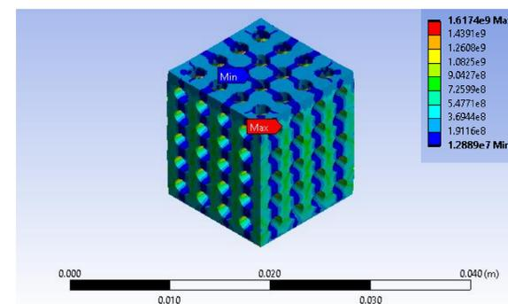
Figure 5: Simulated compression test of Mg foam, stress (Pa)
