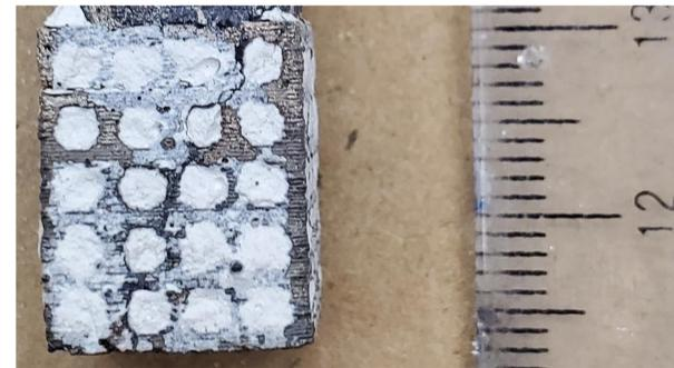
Figure 3: As-cast Mg foam with excess ceramic material
