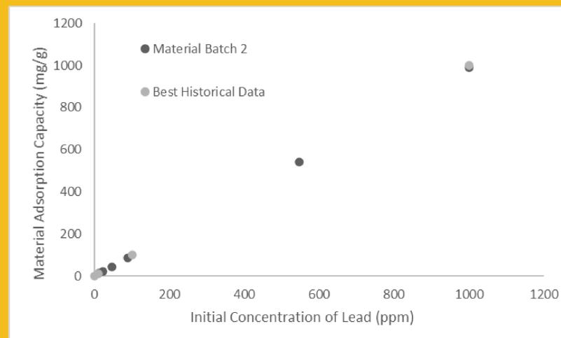
Figure 2: Batch 2 adsorption capacity compared to best historical data
