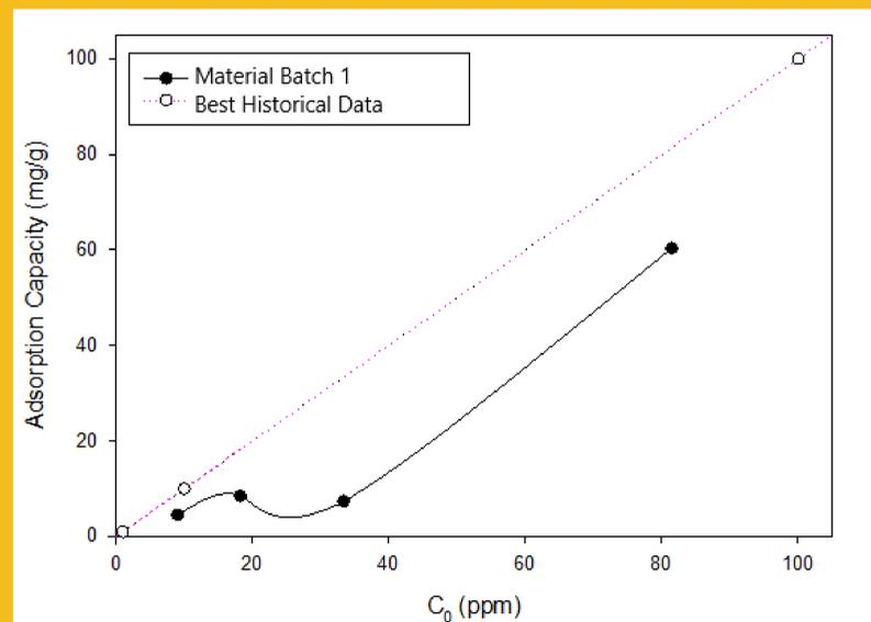
Figure 1: Batch 1 adsorption capacity compared to best historical data
