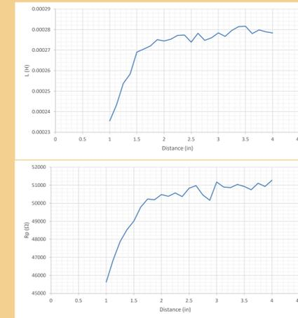
Figure 7: Top: Change of Inductance against target distance, Bottom: Change of parallel losses (Rp) against target distance
