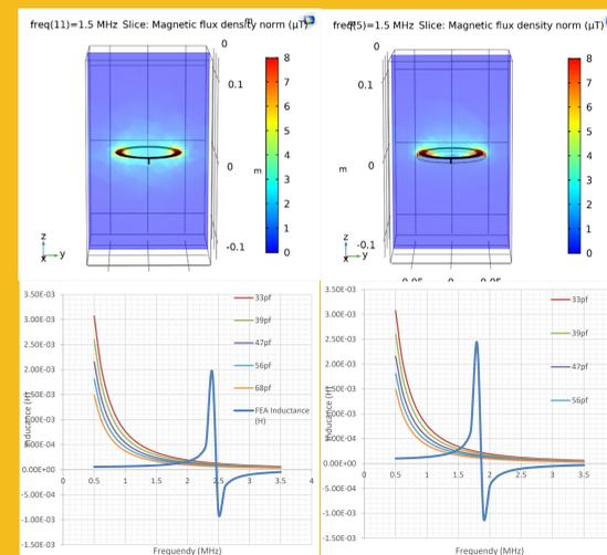
Figure 5: Top Left: FEA without core, Top Right: FEA with core, Bottom Left: Frequency Sweep without core, Bottom Right: Frequency Sweep with core
