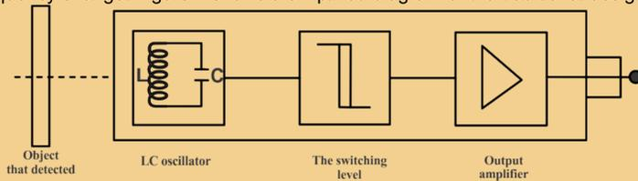
Figure 1: Traditional LC Tank based detection circuit
