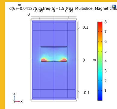
Figure 6: FEA model for parametric sweep with a steel target
