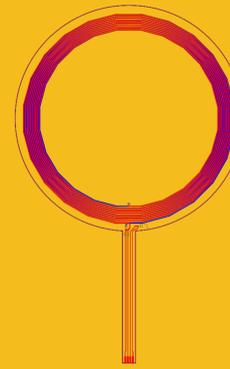
Figure 4: Hollow 2-layer FPC coil with capacitor, NTC Thermistor and edge connector.
