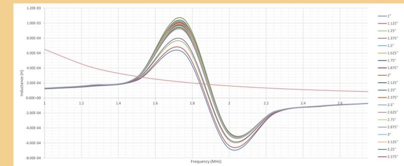
Figure 8: Frequency sweep inductance for each distance superimposed on each other with the LC tank frequency response
