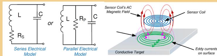
Figure 2: Parallel and Series electrical model of Eddy current losses on a spiral electromagnetic coil
