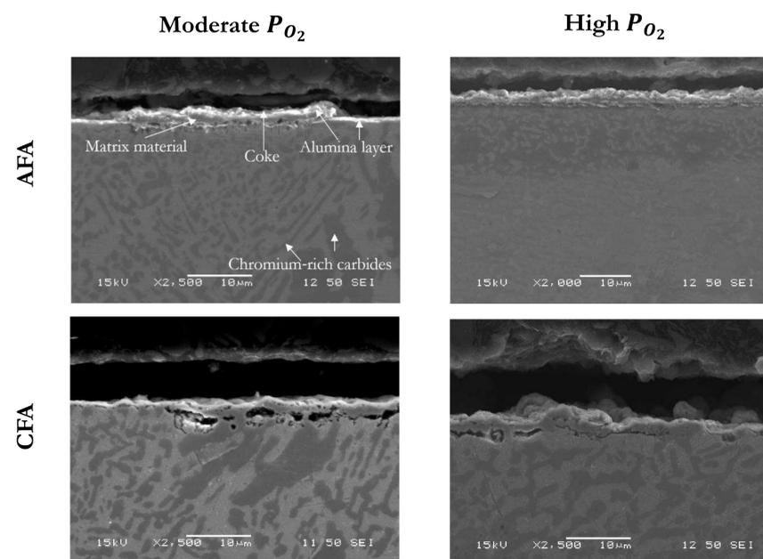
Figure 4: SEM microstructure after each decoking procedure for AFA and CFA alloys.
