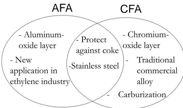
Figure 2: Alumina-forming alloys (AFA) vs Chromia-forming alloys (CFA)
