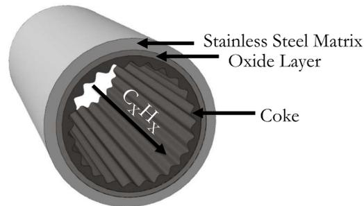
Figure 1: Representation of carbon buildup.
