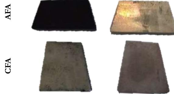
Figure 3: Images of coked and decoked procedure for AFA and CFA alloys.. Scale bar at ~2 cm.
