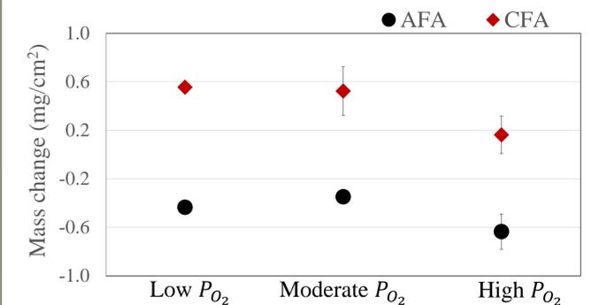
Figure 5: Average change of mass after each decoking treatment. Negative values indicate that mass decreased.
