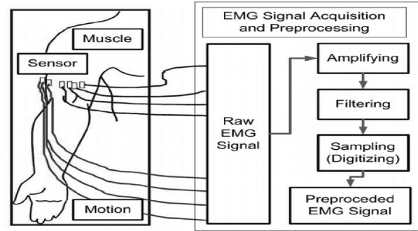
**Figure 3:** Schematic of EMG signal path.
