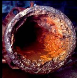
Figure 1 | Late stage biofilm growth in a pipe
