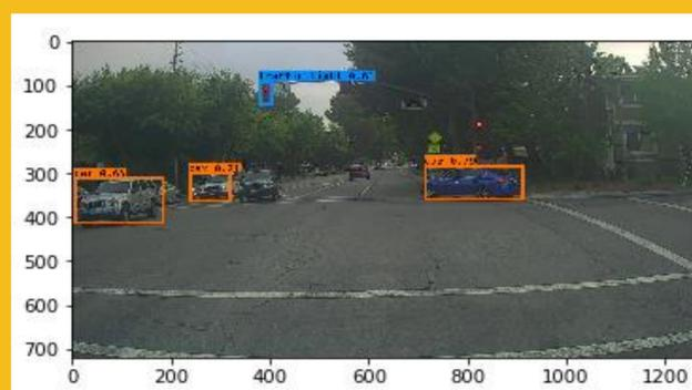
Fig 4: CNN based output of a picture that detects the cars in the streets along with the traffic lights. Note that it detects the traffic light as a whole but not particularities like if the signal on or off for pedestrian crossing. It also misses out on detecting a few cars [1].
