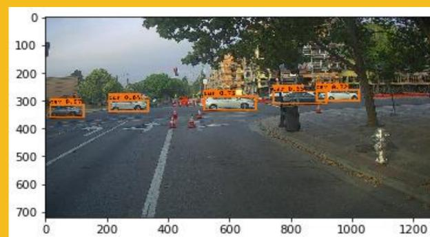
Fig 5: CNN based output of a picture that detects the cars in the streets. Note that this time it detects all the cars in its vision. For pedestrian walkways, challenges increase because it needs to identify the trees, trash cans, etc. Also, the cones in the zebra crossing needs to be recognized [1].
