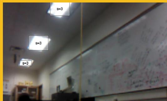
Fig 2: Pixy2 Camera detecting the ceiling lights as trained
