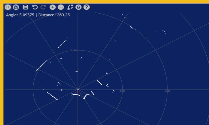
Fig 3: LiDAR sensor mapping the environment in two dimensional. Prints the angle and distance on top left corner.
