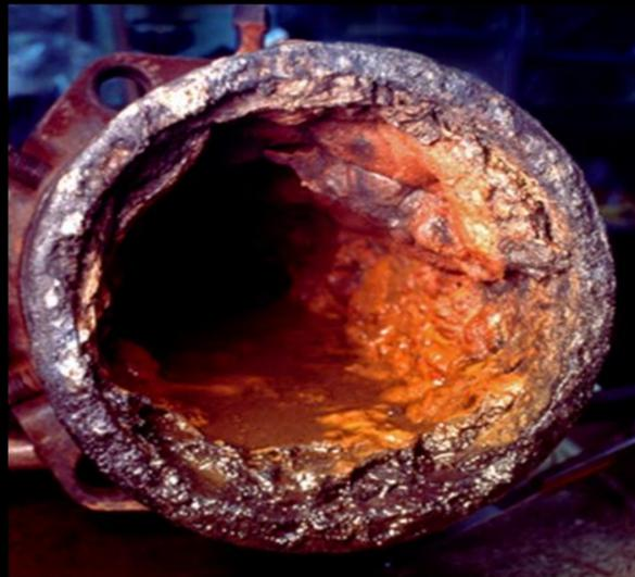
Figure 1 | Biofilms in city water supply pipe.
