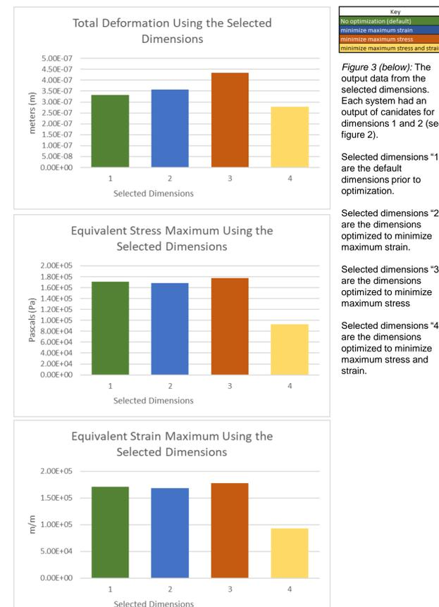
Figure 3 (below): The output data from the selected dimensions. Each system had an output of candidates for dimensions 1 and 2 (see figure 2).
