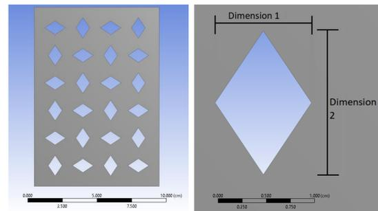
Figure 2 (left): The part created. A close up of the diamond shaped cuts show dimension 1 as the horizontal dimension and dimension 2 as the vertical dimension. The default values for dimensions 1 and 2 are 1 cm and 1.5 cm, respectively.
