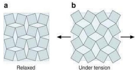
Figure 1 (left): An example of an auxetic structure. The diamond cuts in the material create a structure so that when it experiences tension, the structure expands creating a negative Poisson ratio. This structure is known as kirigami.
