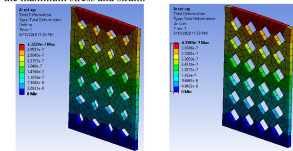
Figure 2 (above): The total deformation simulations of the part. The simulation on the right is prior to optimization and the simulation on the left is the part optimized to minimize the maximum stress and maximize the total deformation. With the optimized geometry, the part is able to deform more with an almost similar stress to that of the default geometry.
