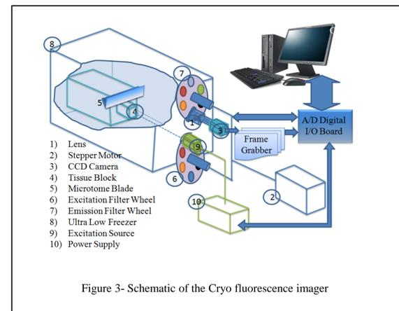
Figure 3- Schematic of the Cryo fluorescence imager
