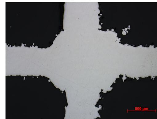
Fig.6: Porosity in struts
