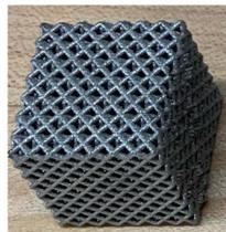
Fig.4: SS316L 3D printed sample
