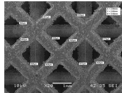
Fig.5: SEM image with cell and strut sizes
