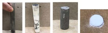
Figure 1A: Graphene and nickel powder in glass tube with graphite coating. 1B: This layer of Zirconia wash on the outside of tube. 1C: Aluminum sample used for infiltration. 1D: Felt circle placed inside glass tube to prevent graphene or Nickel powders from being lost.
